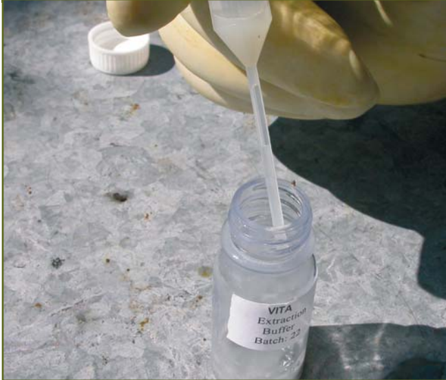
Figure 50: Using a Lateral Flow Device (LFD) A sample of suspect infected larval material is placed in the buffer bottle and shaken for about 20 seconds. 2-3 drops of the resulting suspension are then placed on the lateral flow device. The blue lines at the C (Control) and T (Test) line indicate a positive result for foulbrood infection.
